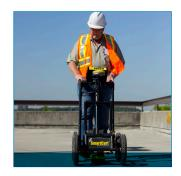
Assess the interior of concrete for deterioration
